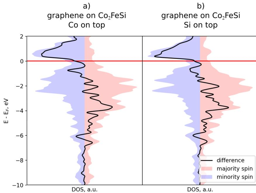
**Fig. 3.** Comparison of densities of states (DOS) for graphene on Co- (a) and Si-terminated (b) faces of Co<sub>2</sub>FeSi.
