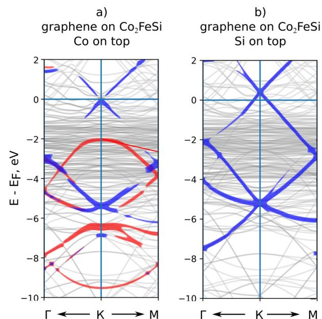
**Fig. 2.** Comparison of electronic structure for graphene on Co- (a) and Si-terminated (b) faces of  $\text{Co}_2\text{FeSi}$ .
