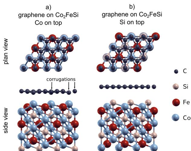
**Fig. 1.** The supercells used for calculation of the graphene/ $\text{Co}_2\text{FeSi}$  electronic structure with graphene on top of Co- (a) and Si-terminated (b) surfaces.
